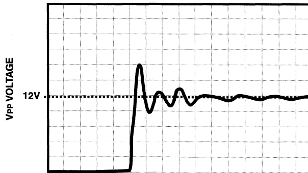
Figure 1 12V SWITCHED BY A RELAY
